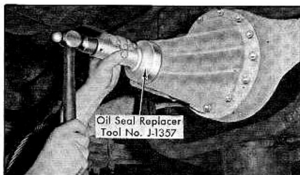
Fig. 8-6 Installing Pinion Oil Seal
